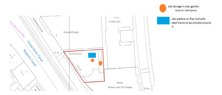
It is proposed to erect a gantry scaffold within the site, where at high level, smaller, higher value items may be stored. Access for existing residents/tenants will be maintained to allow rear access to the rear of the properties.
