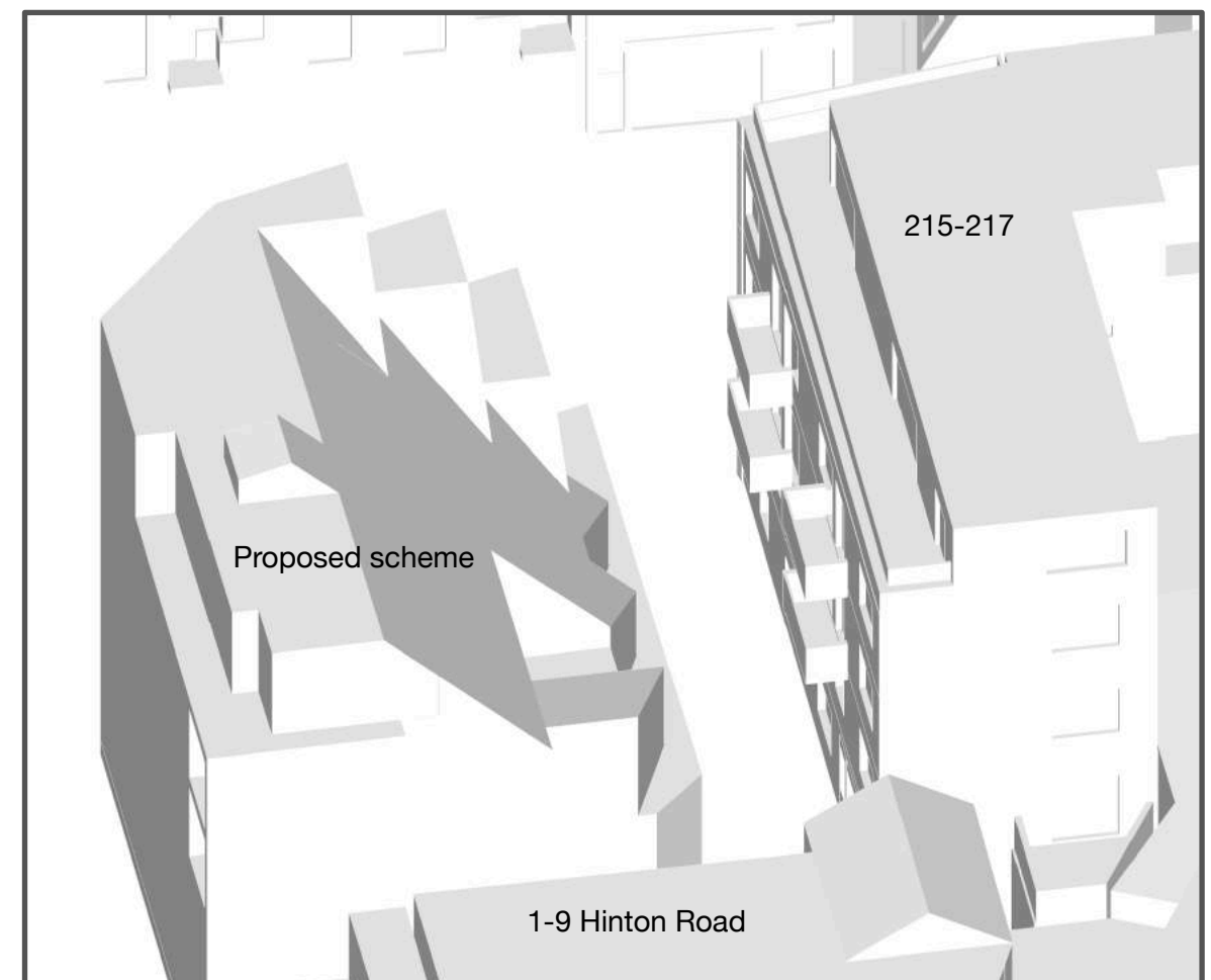
para. D 1.8 High level volumetric view looking NORTH showing raking and stepped roof allowing greater daylighting and better outlook to the adjacent property.
